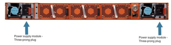
**Figure 2** Connecting AC Power (GigaVUE-HC1)
